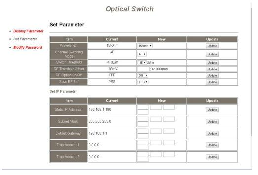
The **Item** shows the changeable parameters, **Current**—the current parameters; **New**—select or enter the new parameters; **Update**—update the parameters.
